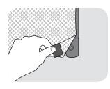
1. Pull back velcro to reveal bolt holes locations on the "Back Assembly."
